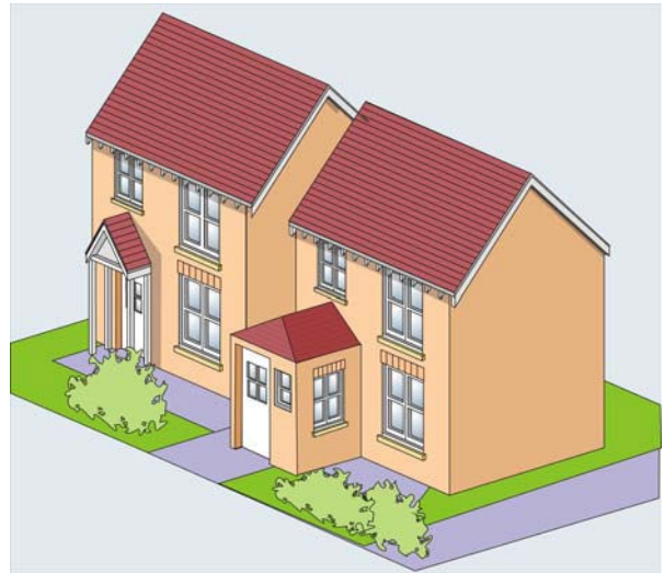
Diagram 8: Inappropriate porch extension.
