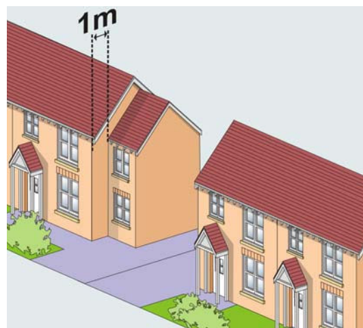
Diagram 10: Good side extension - set back 1m and with lower ridge height
