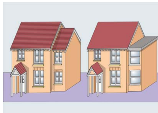
Diagram 2: Examples of side extensions – one with an appropriate pitched roof and well matched windows and one with an inappropriate flat roof and poorly matched windows.
